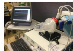
Figure 1: Illustration of the measurement setup, featuring the two side stream sample tubes. One of these belongs to the standard Ecomedics setup, the other is a custom addition and feeds into the ndd device.
